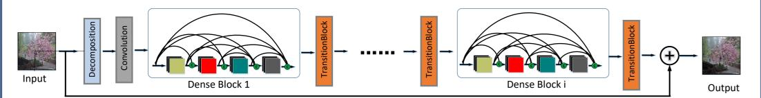
First, the input image is decomposed by guided filtering to obtain high-frequency layers containing rain streaks and image background contours. Then, it passes through
